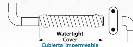
**5.** Vibration Eliminators are most effective when installed perpendicular to the major motion. The fixed end should be securely anchored as close as possible to the Vibration Eliminator. When major motion exists in two planes two Vibration Eliminators should be installed.
