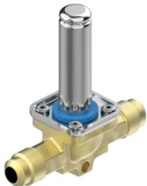
**032F8116****Solenoid valve, EVR 3, Flare, 3/8 in, Function: NC**Body material: Brass, Kv value [m<sup>3</sup>/h]: 0.270, Packing format: Multi pack**PRODUCT DETAILS**
