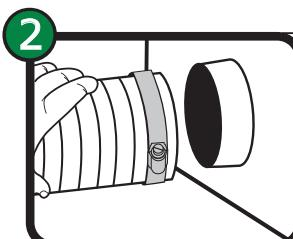
Attach one end of flexible aluminum duct to exhaust outlet pipe using clamp (Not Included) and tighten.
