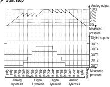
In examples 11 and 12, the step for each digital output is 5 psi (20 psi divided by 4). The conclusion is that each digital stage corresponds to 20% of the analog output (digital output step divided by the analog hysteresis, 5 divided by 25 psi in this case). Thus, whenever the controller activates or deactivates a digital stage, the analogue output will be compensated by being increased or decreased by 20%.
