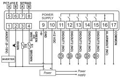
**ELECTRICAL CONNECTION** TRANSDUCER: Brown: 12Vdc
