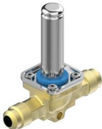
**032F8107****Solenoid valve, EVR 3, Flare, 1/4 in, Function: NC**Body material: Brass, Kv value [m<sup>3</sup>/h]: 0.270, Packing format: Multi pack**PRODUCT DETAILS**
