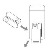
The remote controller is powed by two dry batteries (R03 / LR03 / AAA) X2 housed in the rear part and protected by a cover.
