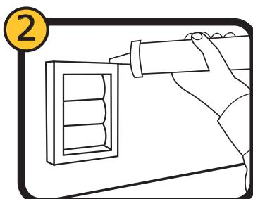
Secure to outside wall using 4 screws (Not Included). Caulk around vent and outside wall if necessary.
