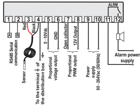
For a current higher than the specified value, use a power relay for activating the alarm.
