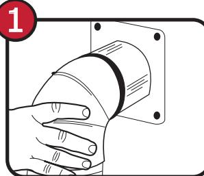
Attach crimped end of aluminum elbow to vent pipe on the interior wall side by pushing into vent pipe opening firmly. Attach the other end of elbow to the crimped end of straight rigid pipe.
