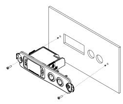
After securing the extension frame with the product, close the side hinges, concealing the screws.
